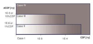
Figure 1: Acceptance Guidelines Considering Core Damage Frequency
